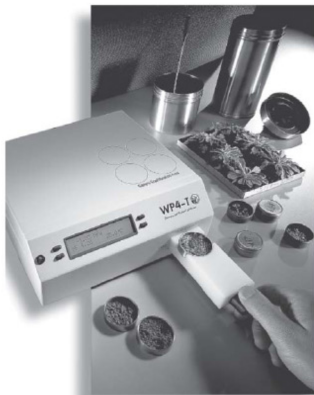
▲ WP4-T —Soil or plant water potential is computed using chilled mirror dewpoint.
