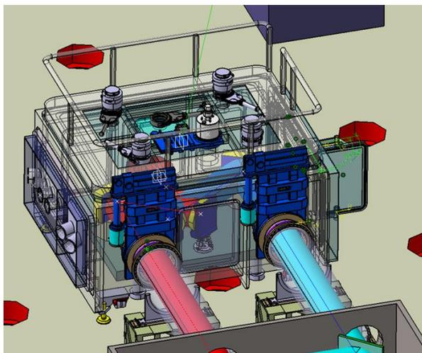
Fig. 4. The E1 Interaction chamber design. The two laser beams are shown in red and blue
