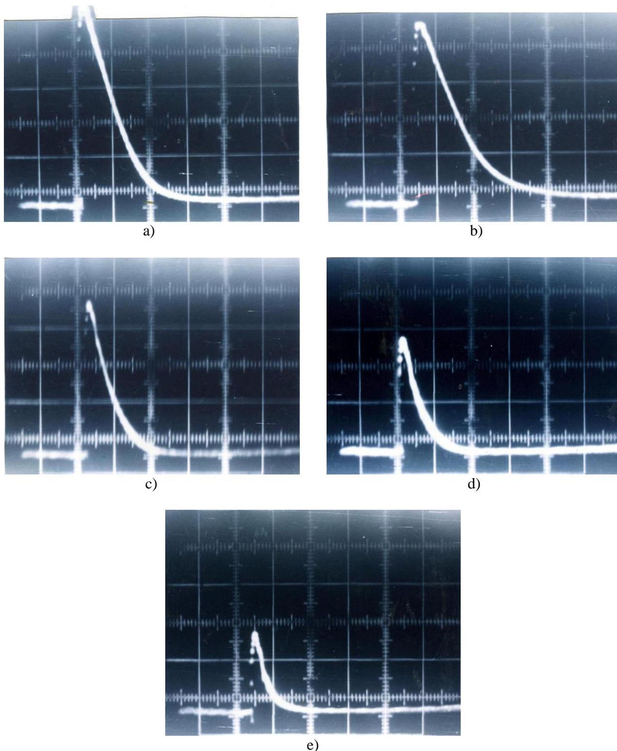
Fig. 2. Relaxation curves of photoconductivity of a thin film of  $ZnS_xSe_{1-x}$  at different temperatures of the sample A.090 ( $d=0.90 \mu m$ ,  $T_{sup}=300 K$ ,  $r_d=1.70 nm/s$ ) (in ordinate is indicated  $\Delta\sigma=\sigma_L-\sigma_0$  in relative units):
