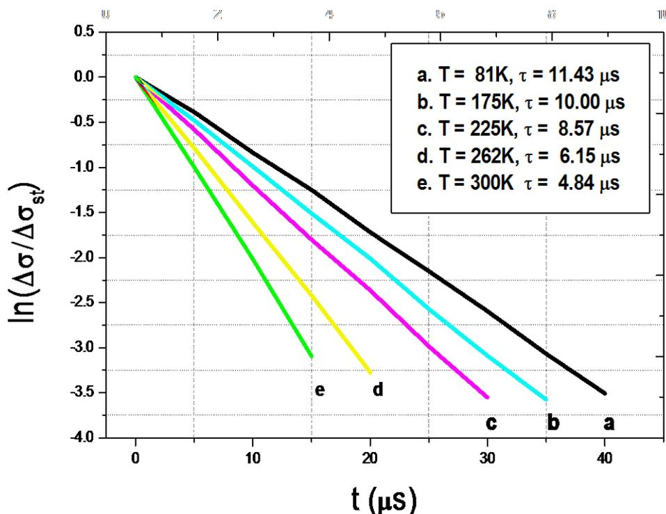
Fig. 3. Dependencies  $\ln(\Delta\sigma/\Delta\sigma_{st})=f(t)$  obtained at different temperatures of the  $\text{ZnS}_{0.5}\text{Se}_{0.5}$  thin film (A.090 sample,  $d=0.90 \mu\text{m}$ ,  $T_{sup}=300 \text{ K}$ ,  $r_d=1.70 \text{ nm/s}$ )
