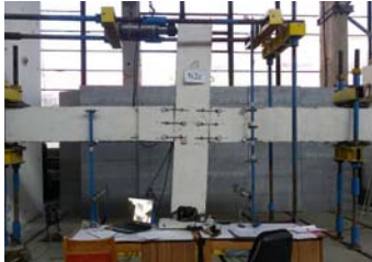
Seismic type loading of modified special hybrid joint specimen
