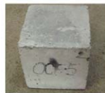
Polypropylene fiber reinforced concrete after exposure to 500 °C
