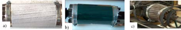
Figure 1. Installations for verification of squirrel-cage rotors: a) flaw detection with active magnetic particle; b) flaw detection with flux detector; c) flaw detection with oscilloscope method
