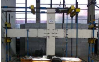
The specimen after test, restoring its initial geometry and with interface cracks virtually closed
