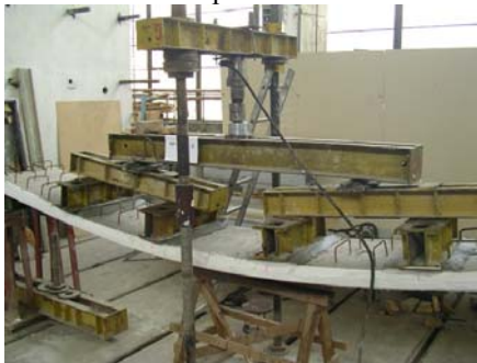
Testing prestressed precast SCC floor element
