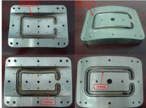
Core and cavity inserts of a new design of conformal cooling channels applied in RHCM
