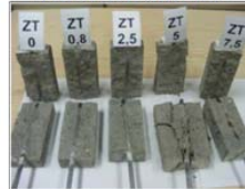
Experimental stand used for electrochemical tests
