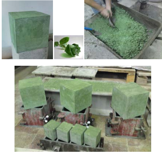
Eco-friendly composite material made of recycled mineral as aggregate and waste glass
