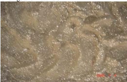
Photo1. A mixture of clay, cement, polyvinyl acetate, polystyrene beads and polypropylene chips
