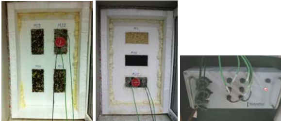
The test stand used to determine the thermal performance of materials.
